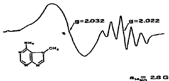
Fig. 7. Experimental ESR spectrum of \text{Fe}(\text{NO})_2(7\text{-CH}_3\text{-adenine})_2 at \text{pH} = 5.5 ( g = 2.022 ).
